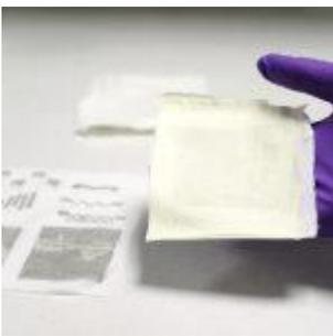
A crucial component in the fabric is a polymer that, when pressed or squeezed, converts mechanical stress into electrical energy. It is also made with stretchable spandex as a base layer and integrated with a rubber-like material to keep it strong, flexible, and waterproof.
